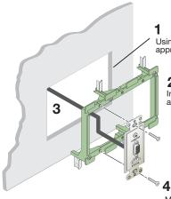
Using the supplied mud ring as a guide, mark and cut out the appropriate material within the marked area.
